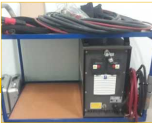
Induction Heater for Mounting Bearing (melepaskan dan memasang bearing)
