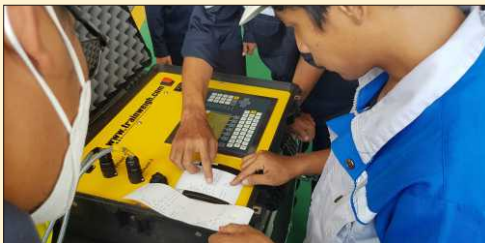
Wheel Weighing Device Berkfungsi mengukur berat beban sarana
