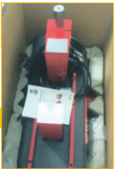
Heater for dismounting of roller bearing inner rings (melepas bagian dalam bearing)
